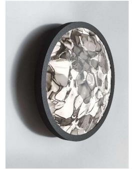
**Tech. description** The light comprises a milled dural body with integrated LED module and balancing system and a mounting bracket. The Brokisglass shade is attached to the body of the light via bayonet system. The light is intended for installation on a wall or ceiling.
